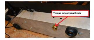
WARNING: There is no need to adjust torque knob starting since Lynx II. It is actually replaced by a plug.
